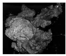
Sandy, Metallic Grease Sample Recovered from the Ends of the Jackscrew of N963AS
