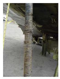
Jackscrew from N963AS, Recovered without any Grease on the Operating Surfaces and with Remnants of Screw Shavings Still Attached
