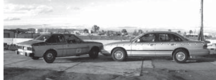
Figure 1: Position of the target vehicle (left) and bullet vehicle (right) prior to impact
